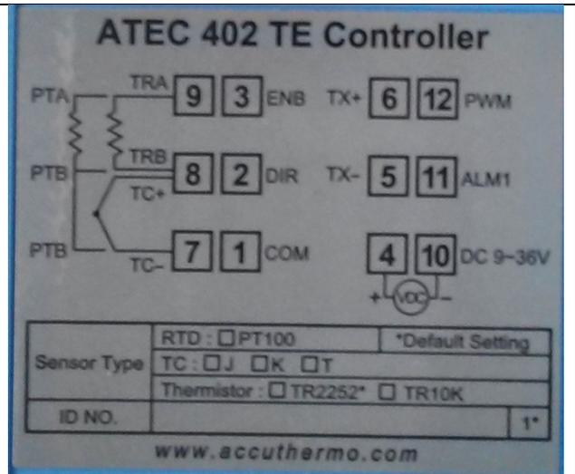
The new ATEC402 has 4-plugable connector with number mark on it. This make wiring connection much easier.
